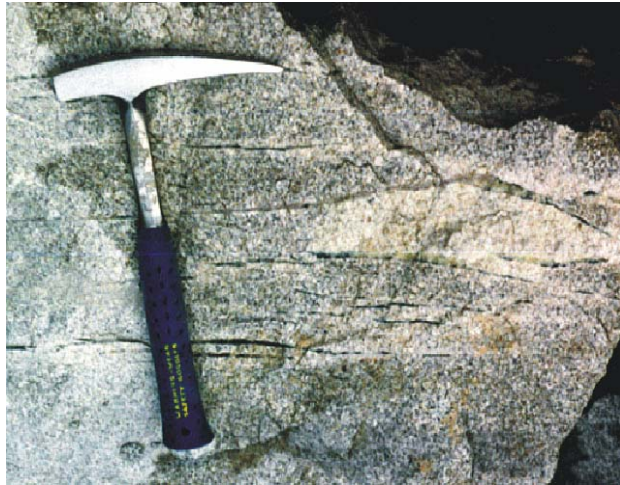
Fig. 3. Example of granite cut by multiple hydrothermal veins of different thickness.
