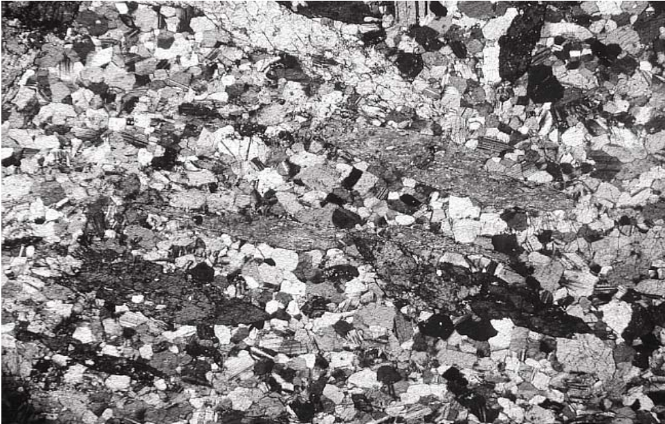
Fig. 4. Fine-grained variety of the hornblende-bearing “grey” plagiogranite from northern part of the Szklary massif; crossed nicols, magn. 25×.
